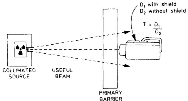
*The transmission factor as an indication of the effect of the primary barrier.*
