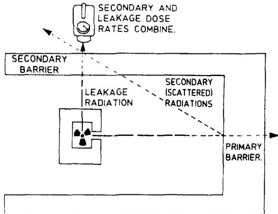
*Secondary barriers are used to shield secondary radiations.*
