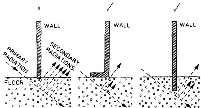
*Methods to prevent radiation scattering under a wall.*
