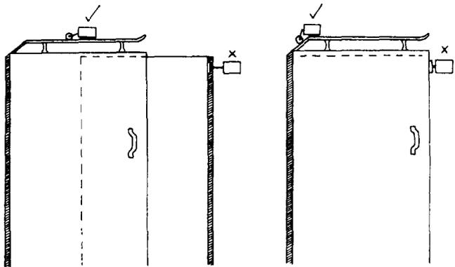
*Fail-to-safety installation of a door interlock:
